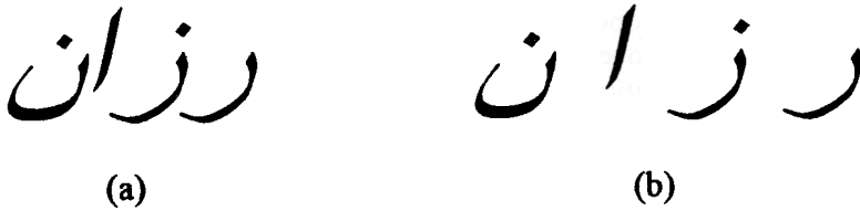
FIG. 1. An Arabic word with overlapping (a), and the same word after overlapping is resolved by a shifting process (b) [2] .
